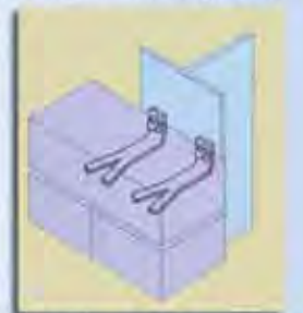
Brickwork fixed tie
