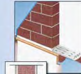
Internal steel lintel
